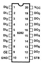
Figure 1. 8282 Pin Configuration
